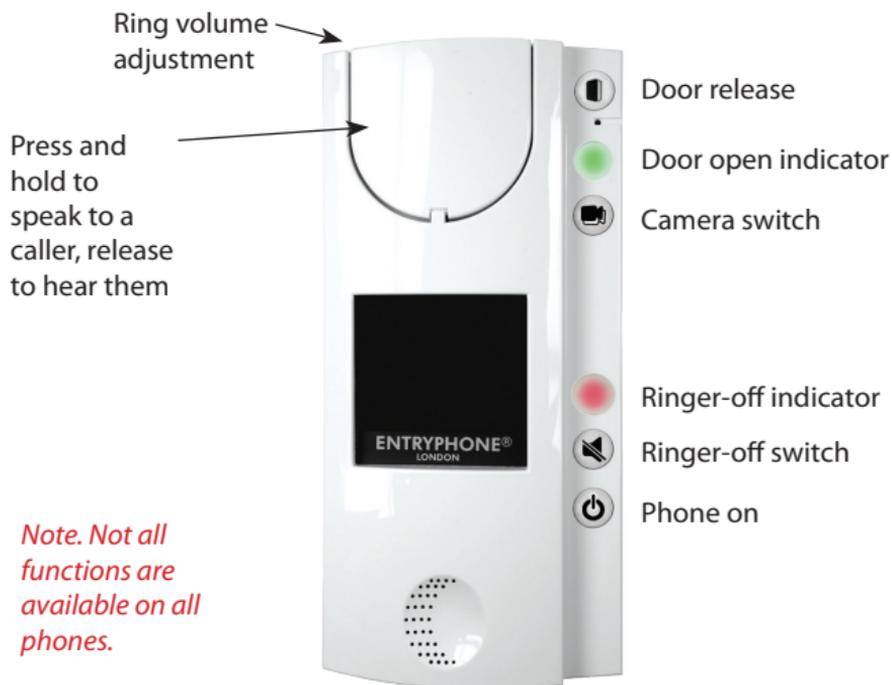
The Entryphone 501PTSP# is a wall-mounted, colour video, loudspeaking telephone. There is the large speech operation button on the top and smaller function buttons and indicator lamps along the right hand side of the unit.
