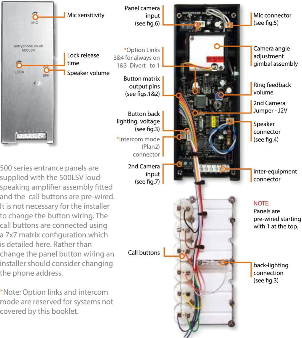
500 series entrance panels are supplied with the 500LSV loud-speaking amplifier assembly fitted and the call buttons are pre-wired. It is not necessary for the installer to change the button wiring. The call buttons are connected using a 7x7 matrix configuration which is detailed here. Rather than change the panel button wiring an installer should consider changing the phone address.
