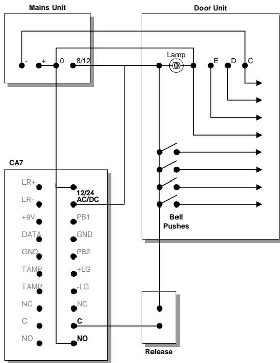
The CA7 shown above connected with Entryphone® plan 1. Only Relay 1 is shown used.
