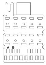
At manufacture the buzzer connections are solderd to terminals A and B on the rear of the sub chasis. When replacing either re-solder or connect wires via screw terminals on the front of the sub chasis.
