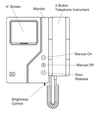
Automatic Operation: In normal operation, the monitor will be activated and stay on for about 90 seconds by a caller pressing the call button on the entrance panel.
