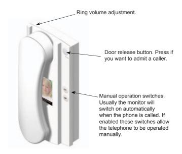
The Entryphone 200V is a wall mounted, colour video, telephone. There are three buttons, the button at the top right operates the door release and the lower "On" and "Off" buttons allow manual operation of the monitor.
