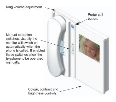
The Entryphone 200V4 is a wall mounted, colour video monitor telephone. There are three buttons, on the telephone, the button at the top calls the porter and the lower "On" and "Off" buttons allow manual operation of the monitor.
